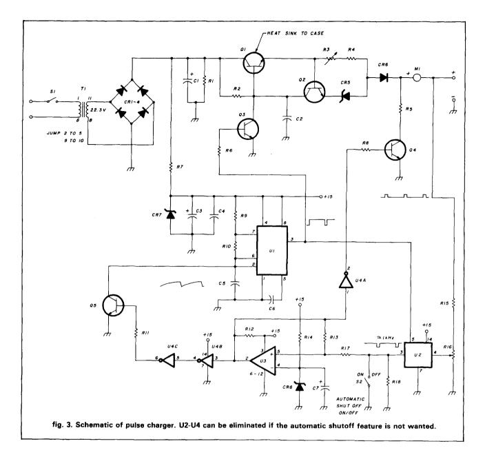
Although pass transistor Q1 is heat-sinked to the case, it must be electrically insulated from it. During conduction, the current through Q1 can be as high as 5 amperes and the voltage across it about 15 volts. Instantaneous power is  $5 \times 15 = 75$  watts, but the power which must be dissipated by Q1 is only ten percent of that because of the duty cycle. Using the case as a heat sink works well for this low power level.
